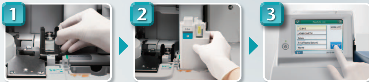
Set the slide (Dry Slide Reagents)
